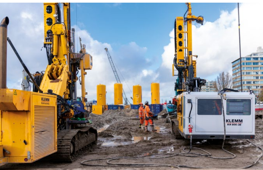
The electric anchor drilling rig KLEMM KR 806-3E gave a convincing performance in a direct comparison on the construction site.
