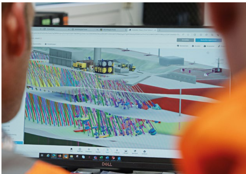
With the help of the 3D model, the geometry can be mapped along with injection volume and pressures.
