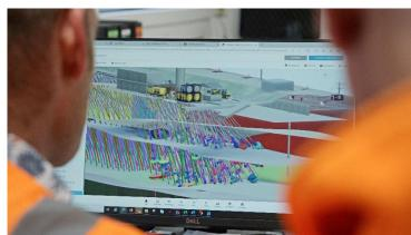
(3) Using the 3D model, it is possible to map the geometries along with injection volumes and pressures.
