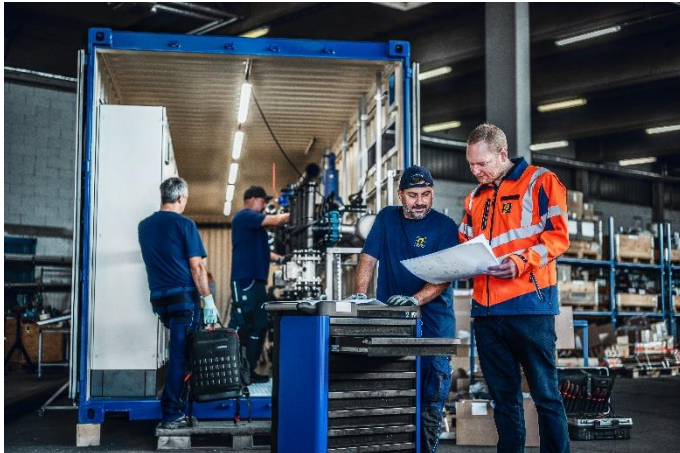
(2) The groundwater treatment plant was customized for the requirements of this project down to the smallest detail and fabricated in the Schrobenhausen plant
