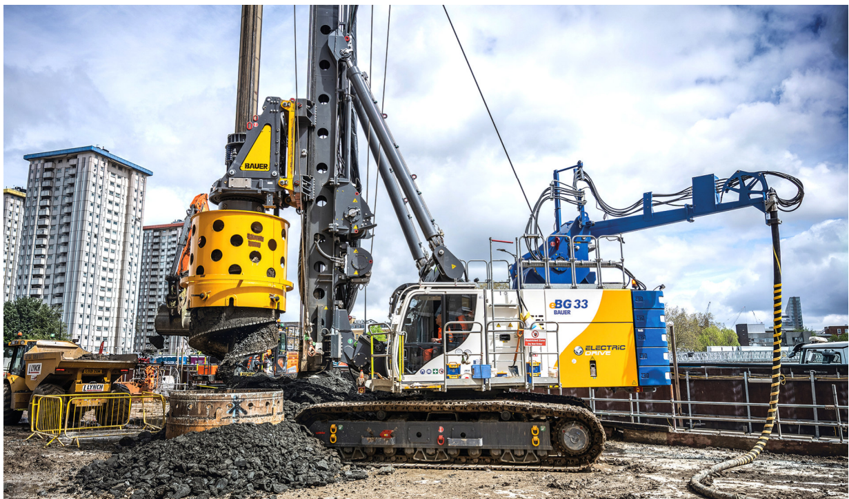
The eBG 33 is the world's first electrified large rotary drilling rig from Bauer.
