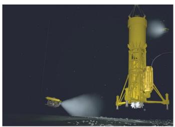
(2) In the "Vertical Approach", the template and diaphragm wall cutter are lowered via a winch instead of being placed once and then moved horizontally along the seafloor.
