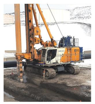
(2) Amongst others, a multi-purpose BAUER BG 30 drilling rig with special Arctic equipment was used.
